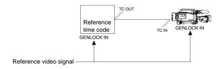
Example 2: When a multiple number of AJ-SDC915 units are connected with one unit serving as the master unit and the others as the slave units
